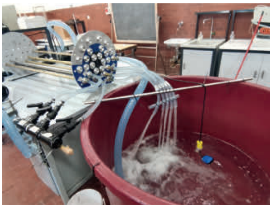
Figure 8. Test setup for seawater flow simulation in coated and uncoated tubes.
