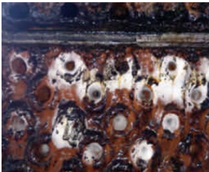
Figure 13. Uncoated tubes bundle after 4 years in the same operating conditions.
