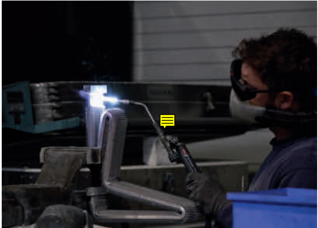
▲ Welder at work on a skived aluminium profile during assembly. Image courtesy of SAG.
