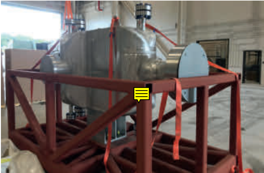
▲ The Heatric "Main Cooler" PCHE after on-site delivery to the 10 MWe STEP Demo project in San Antonio, Texas.
