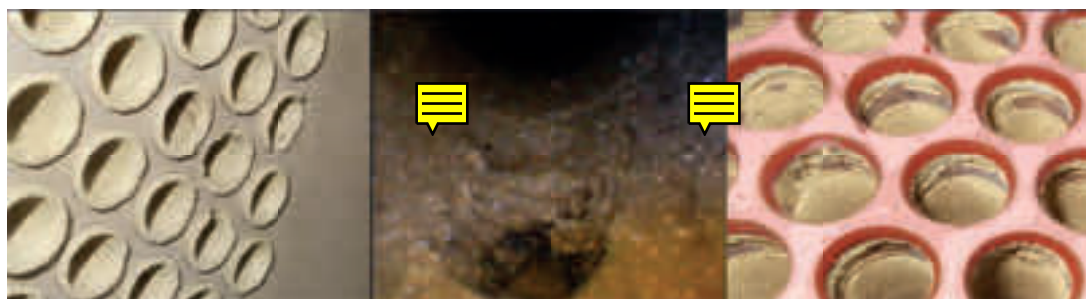
Figure 1. Erosive phenomena related to over velocity in combination with particles in Al-brass/copper tubes.
