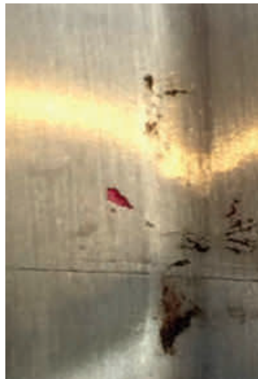
Figure 12. Beginning of corrosion attack.
