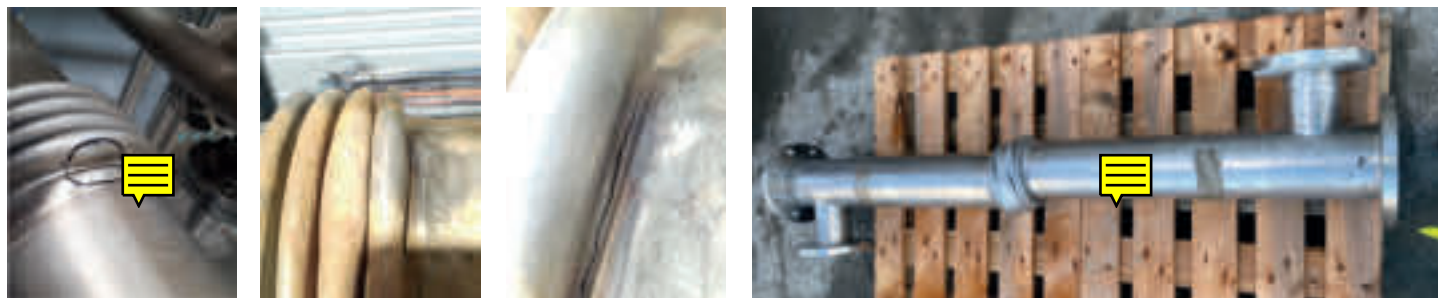
Figures 2, 3, 4 and 5. Examples of expansion joints collapsed and cracked by an overpressure in shell side.
